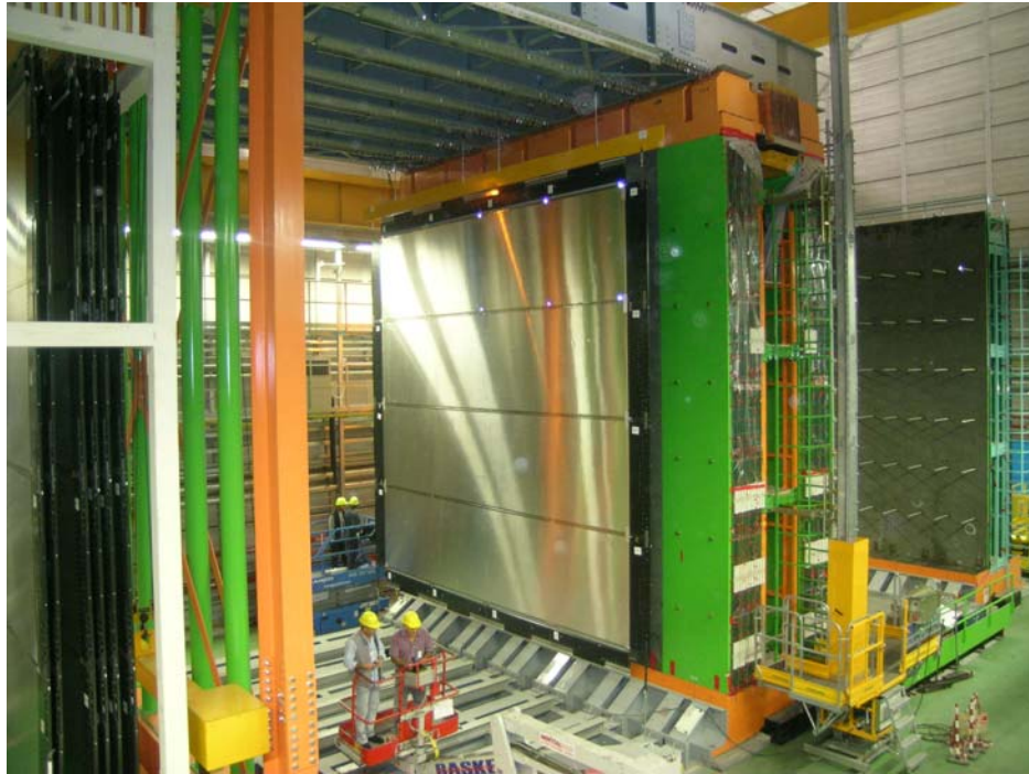
The OPERA detector during construction in hall C of the LNGS underground laboratory in December 2004. In the foreground, the storage arch supports six scintillator strips target trackers. A first tracker is installed in front of the dipole magnet of the muon spectrometer in the empty volume that will host the target of the first super-module. The second magnet is being constructed in the rear.
