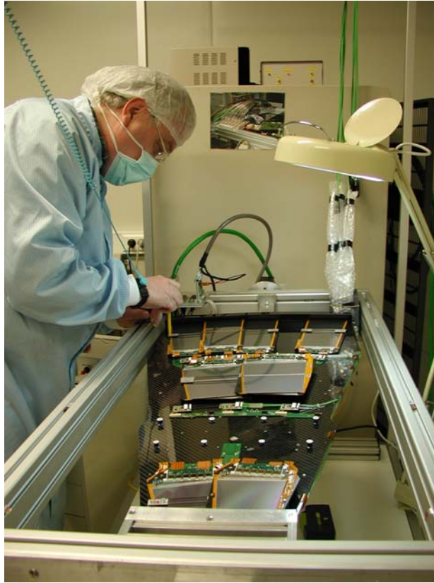
Assembly of the first production petal in the CMS clean room.
