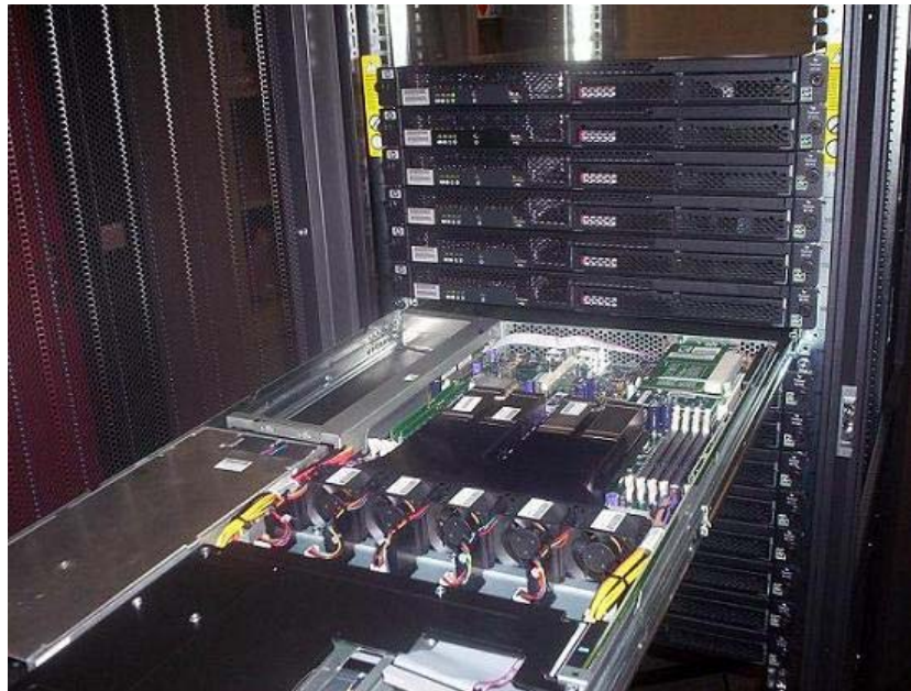
Partial view of the computing nodes (Opteron 64 bits dual processors) of the new grid infrastructure of the IIHE.
