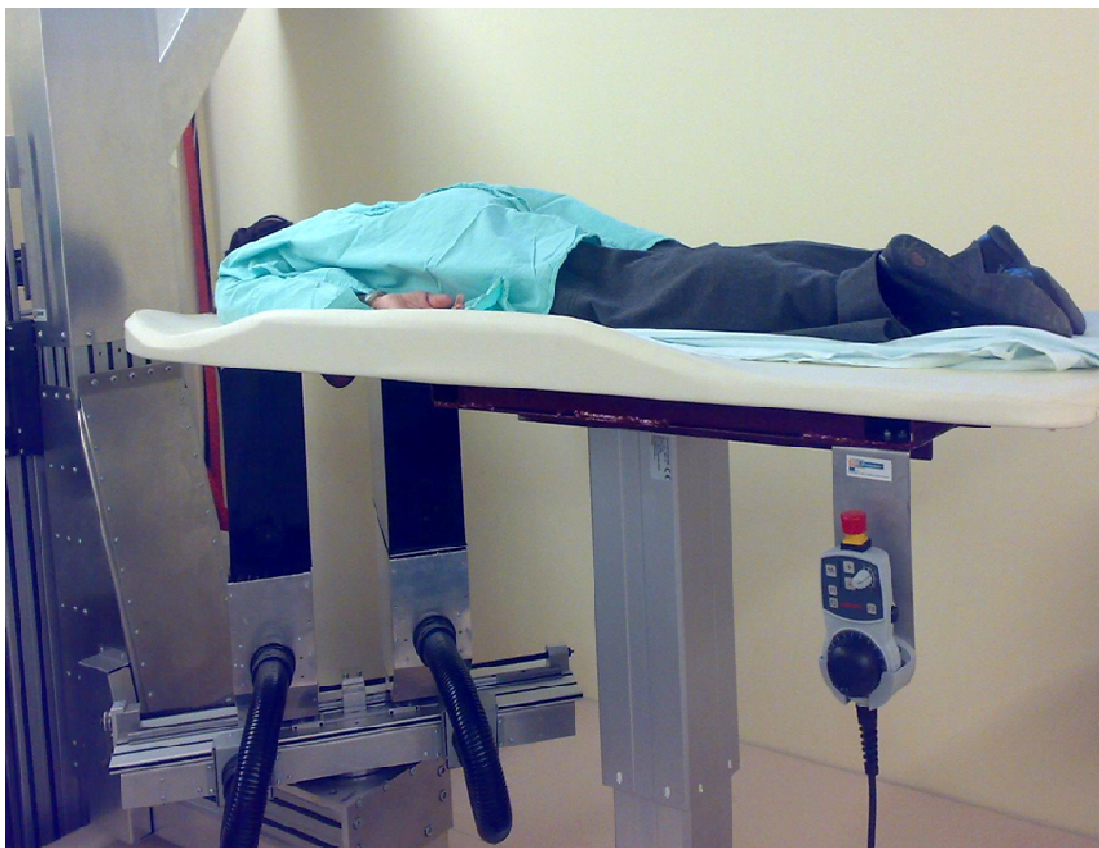
First patients test with the prototype dedicated PET scanner for mammography.
