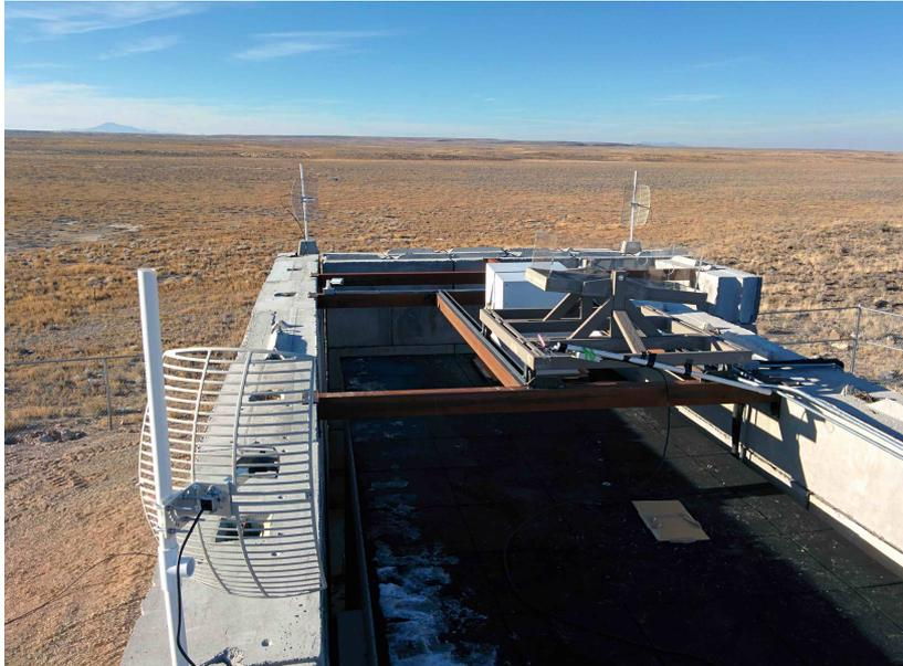
Figure 11: The Radar test array centered around the linac beam hole. The wooden mount is for the ice block.
