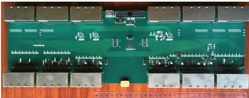
Figure 8: Second version of the JUNO Back-End Card (BEC) built at the IIHE. At the top and the bottom of the board, the ethernet connectors (RJ45) are visible, together with the equalizers. At the centre of the board, the translators and drivers are displaced. The main connector for the mezzanine card for the FPGA is placed at the top centre of the board.
