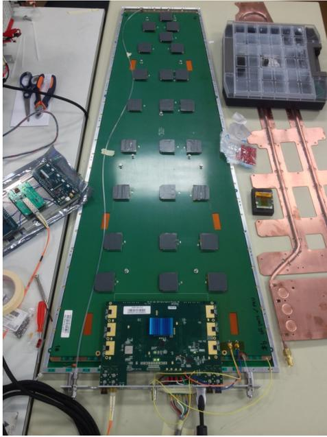
Figure 3: One of 10 Triple-GEM prototypes before its installation in CMS during the 2016-2017 LHC shutdown. The detector is equipped with its new electronics. The opto-hybrid board designed at the IIHE is located on the long base of the detector.
