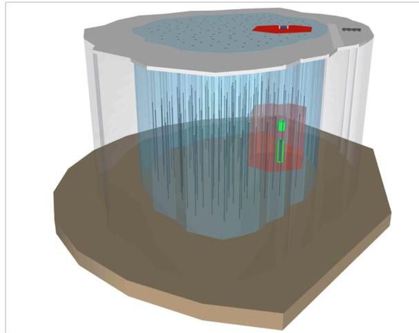
Figure 7: A possible *IceCube-Gen2* configuration. IceCube, in red, and the infill subdetector DeepCore, in green, show the current configuration
