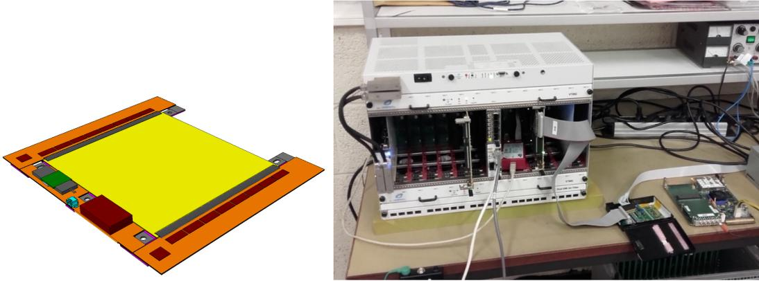
Figure 4: Left: Schematic view of a  $10 \times 10 \text{ cm}^2$  module of the type that will be assembled at the IIHE. Right: Migration from a table-top GLIB board to a data acquisition based on a  $\mu$ TCA crate housing an FC7 board.
