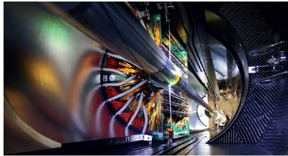
Figure 2.13: The pixel barrel being re-installed after the Long Shutdown in 2015, around the beam pipe at CMS. Picture taken from [102].
